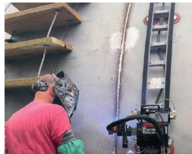
Pipeliner mounted on a stainless steel vessel using vacuum cup kit
