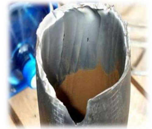
Stress Corrosion Cracking
